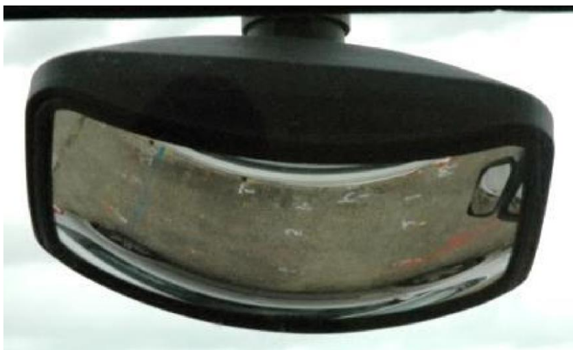
Figure 23. The view that a driver has of a Class V 'Look Down' mirror showing a silver car adjacent to the cab
