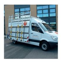
Designed to transport sheets of glass up to 3,215mm x 2,540mm in size
