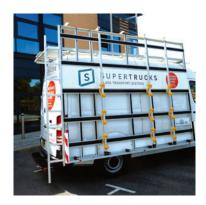
Fitted with roof racks with drop-down ladders at the rear
