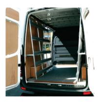
Fitted with two interior racks – one that runs the entire length of the body and a shorter one
