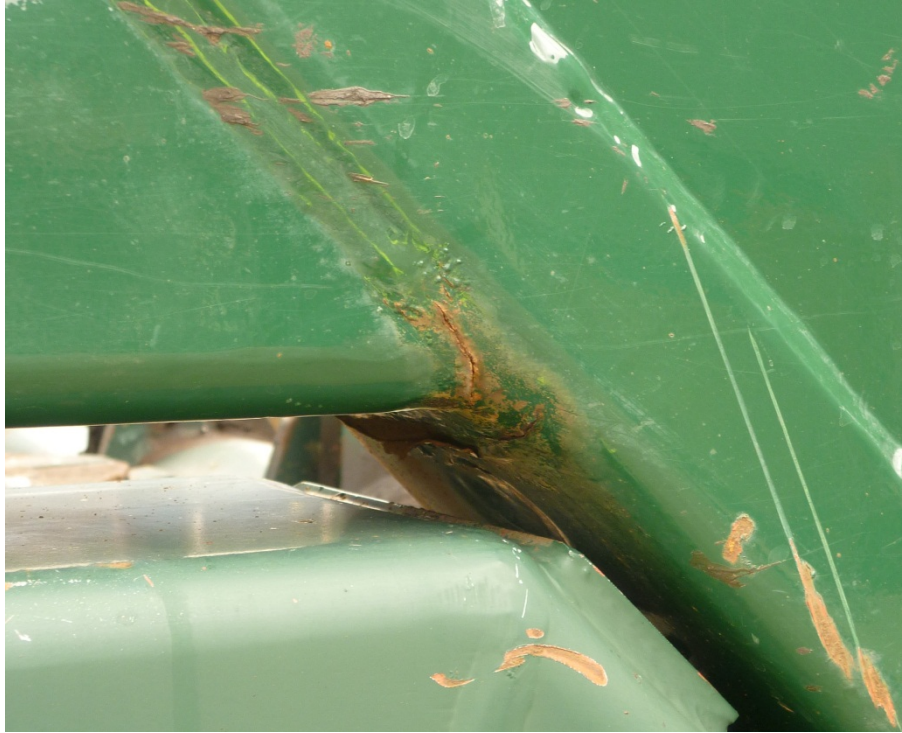
Figure 10 – Crack in lifting arm
