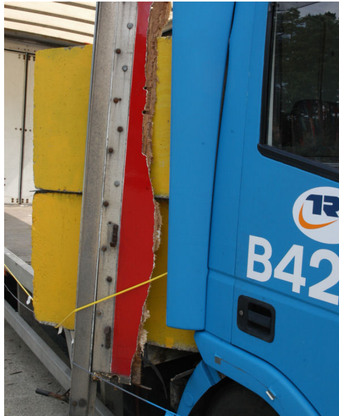
Figure 15 – Damage to headboard (Image supplied by TRL Ltd)
