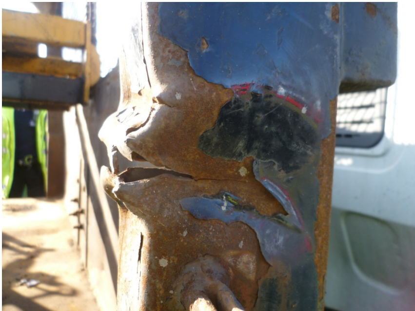
Figure 7 – Damage to headboard upright
