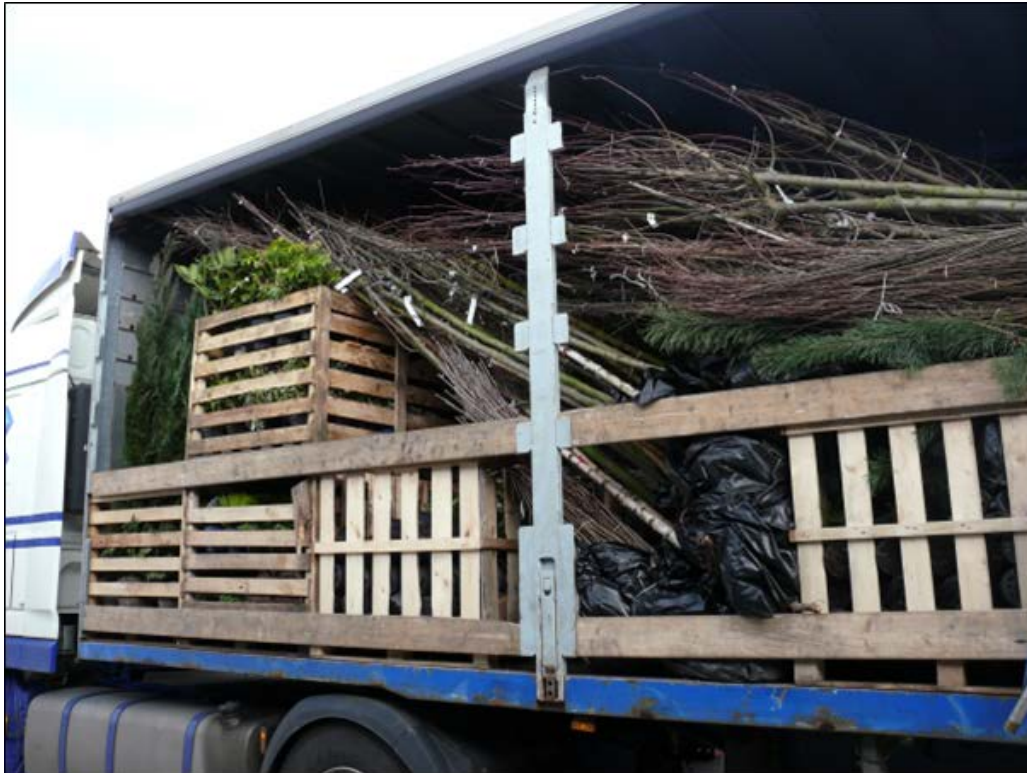
Figure 5 – Curtain-sided vehicle with no load securing
